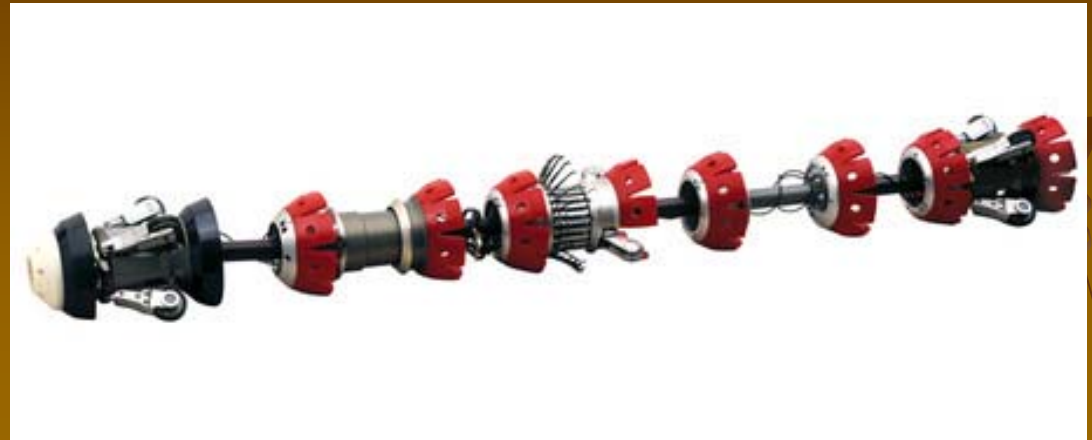
Precision Pipeline Locator – utilized in areas of AC interference for location, depth, current measurement and current direction.
